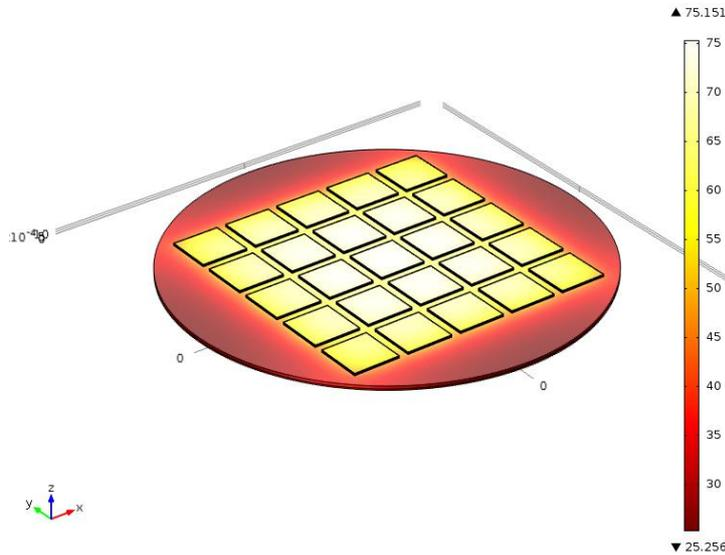
**Fig. 8:** Temperature distribution ( $^\circ\text{C}$ ) of the densely packed receiver under  $500\times$  concentration, convective heat transfer coefficient of  $3.5\text{kW/m}^2\text{K}$  and ambient air temperature of  $25^\circ\text{C}$ .
