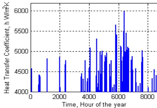
**Fig. 1:** Heat transfer coefficient needed for a maximum cell surface temperature of 80°C.
