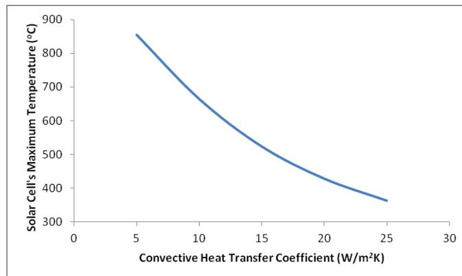
**Fig. 4:** Solar cell's maximum temperature versus the natural convective heat transfer coefficient under 500x suns and 25°C of ambient temperature.
