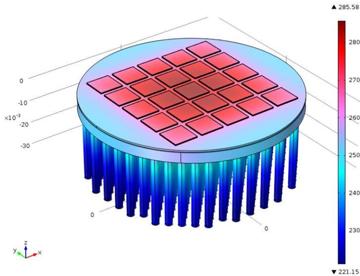
**Fig. 7:** Temperature distribution ( $^\circ\text{C}$ ) of the densely packed receiver under 500x concentration, convective heat transfer coefficient of  $15\text{W/m}^2\text{K}$  and ambient air temperature of  $15^\circ\text{C}$ .
