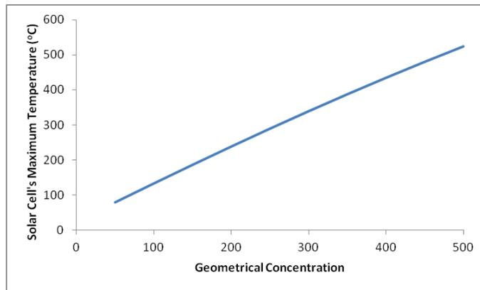
**Fig. 6:** Solar cell's maximum temperature as a function of the geometrical solar concentration and a convective heat transfer coefficient of  $15\text{W/m}^2\text{K}$  and  $25^\circ\text{C}$  of ambient temperature.
