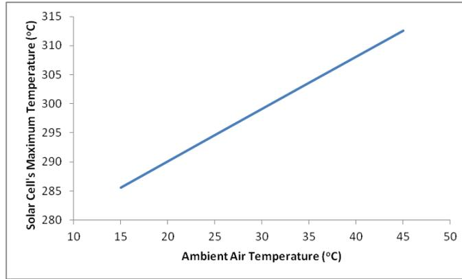
**Fig. 5:** Solar cell's maximum temperature as a function of the ambient air temperature and a convective heat transfer coefficient of  $15\text{W/m}^2\text{K}$  and geometrical concentration ratio of 500 suns.
