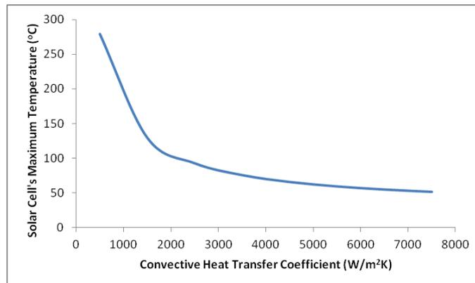
**Fig. 9:** Solar cell's maximum temperature versus the forced convective heat transfer coefficient under  $500\times$  suns and  $25^\circ\text{C}$  of ambient temperature.
