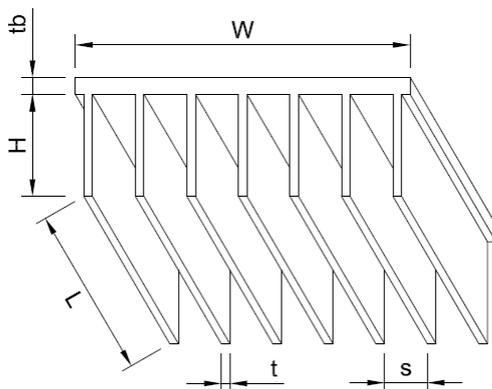
**Figure 1:** Geometric parameters in the developed plate fin array
