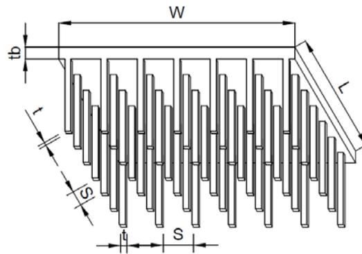
**Figure 2:** Pin fin array design (referred in the text even as "crossed array")
