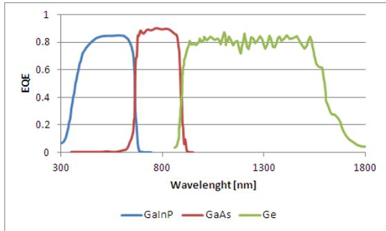
**Figure 9:** EQE vs. wavelength (adapted by Azurspace datasheet)
