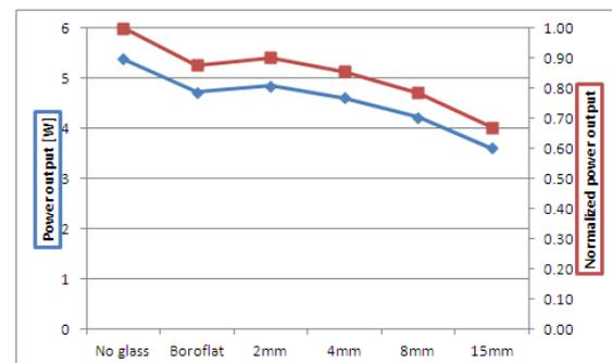
**Figure 12:** Power outputs of the cell with different coverglasses
