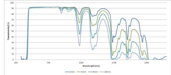
**Figure 3:** Transmissivity values for different PMMA samples
