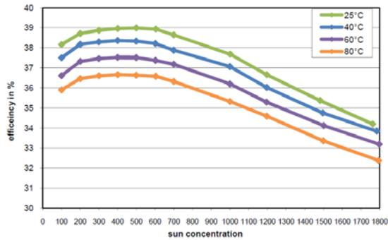
**Figure 2:** Cell efficiencies vs. sun concentrations
