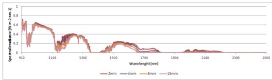
**Figure 6:** The solar spectral irradiances for different PMMA samples
