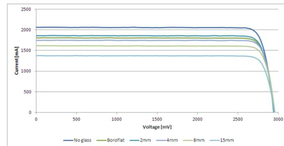
**Figure 11:** I-V curves of the cell with different coverglasses
