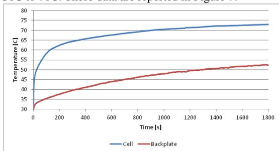
**Figure 7:** Difference in temperature between the cell and the backplate
