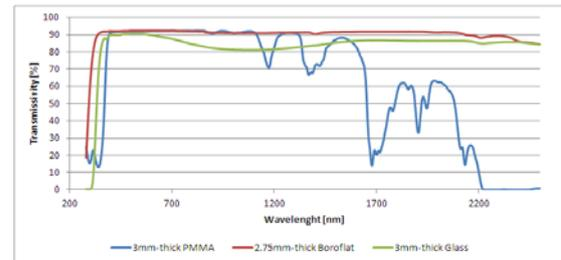
**Figure 4:** Comparison between PMMA, Borofloat and common glass transmission spectra
