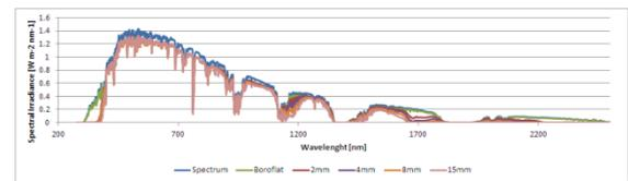
**Figure 5:** AM1.5 solar spectrum and the irradiances through the Borofloat and the PMMA samples
